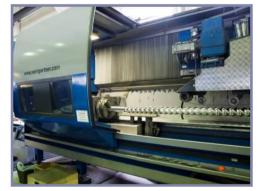
FINISH 450 polishing multiaxis machine tool
